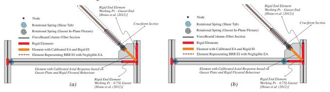
Figure 9: Improved Numerical Model Proposed for (a) Continuous Beam Detail, and (b) Stub Beam Detail
