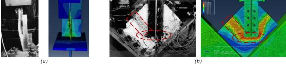
Figure 3. Experimental Results vs. FE Models (a) Specimen MP3A, and (b) Specimen MP1 (experiments from Yam and Cheng [16])
