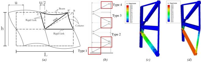
Figure 6. (a) Schematic Illustration of the Modelled Portion using the approach by Kaneko et al. [31], (b) BRBF Illustrating the Gusset Types, (c) S-Shape Buckling Deformed Shape for Type II, (d) U-Shape Buckling Deformed Shape for Type II
