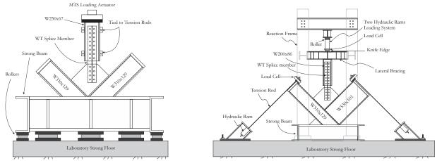
Figure 1. Experimental Setups for Tests Reported by Yam and Cheng [16]
