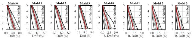
Figure 10: MCE-Level Response for all Models; Transient Drifts and Residual Drifts
